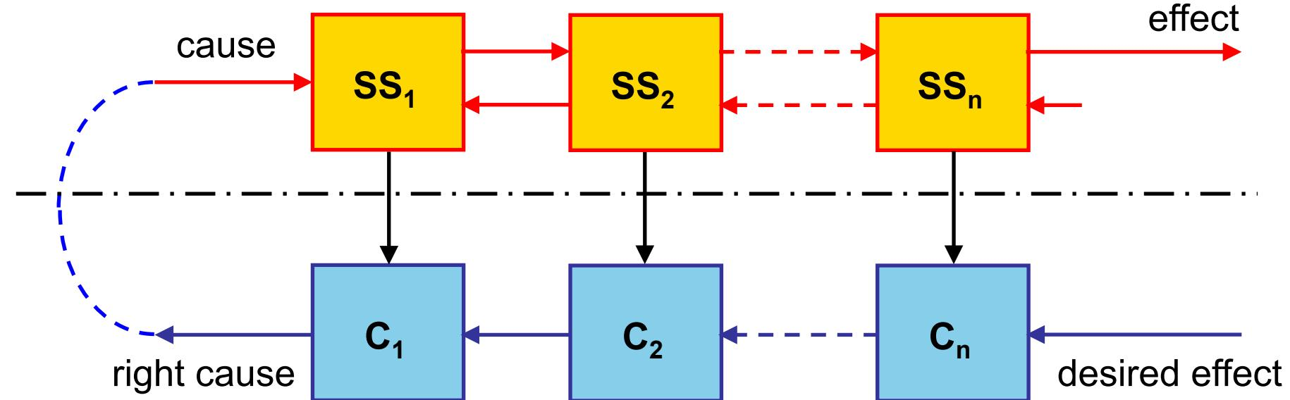
The control scheme is developed as a mirror of the model
