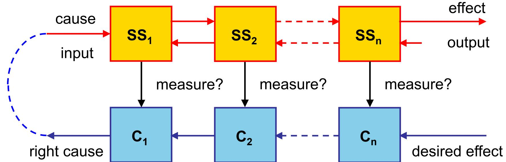
**EMR** = system decomposition in basic energetic subsystems (SSs)
