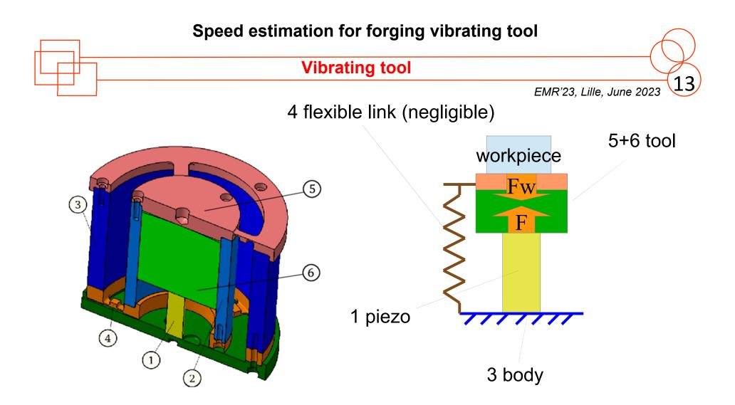
The waveforms must be controlled, but the sensors are too expensive : estimator
