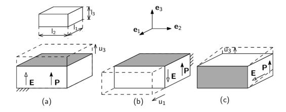
Coupling : direction of deformation w.r.t direction of applied field
