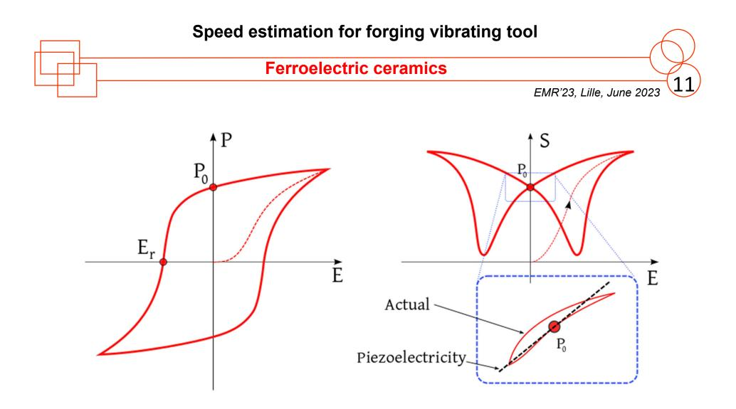
Hysteresis in ferroelectric ceramic : Piezoelectricity is an approximation A closed loop is required to control the waveform
