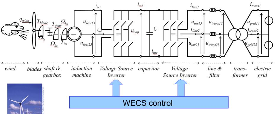
Technical requirements: - provide the maximum active power P - control the reactive power Q
