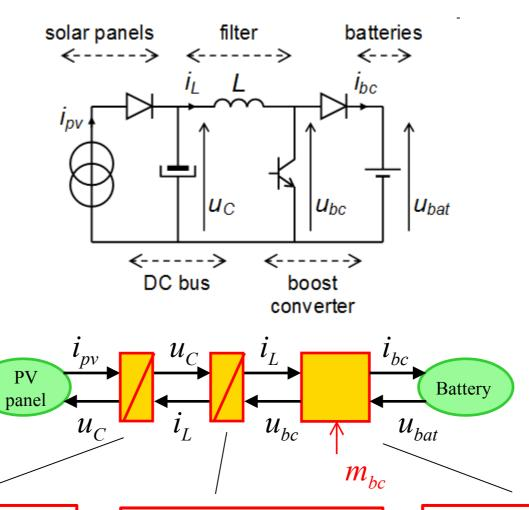
$$C\frac{d}{dt}u_C + \frac{u_C}{R_C} = i_{pv} - i_L$$
