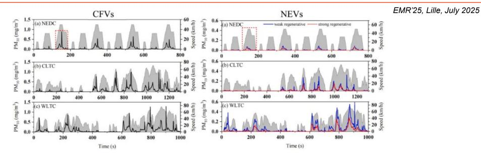
Mass concentration emission characteristics of BWP from CFVs and NEVs under standard test cycle [Zhang 2024]
