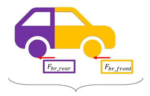
Industrial choice: fix distribution of braking between front and rear brakes: 70% at front and 30% at rear
