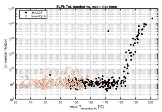
Particle [6nm-10µm] number emissions and average disc temperature for several driving cycles [Mathissen 2018]
