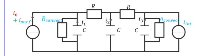
$$\frac{\phi_{convect\_surf} = h(\boldsymbol{v}_{\boldsymbol{v}eh})S(T_1 - T_{ext})}{\phi_{convect\_int} = h(\boldsymbol{v}_{\boldsymbol{v}eh})S(T_3 - T_{ext})}$$
